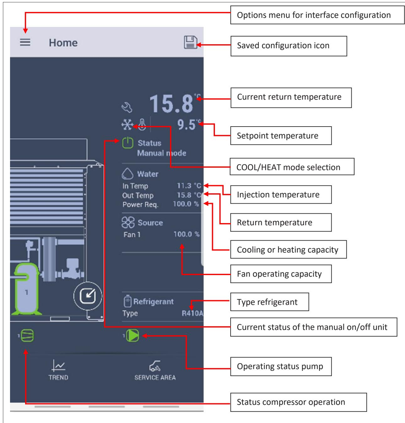
**NOTE:** The microchiller controller cannot be used in tandem units.
