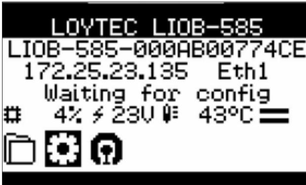
After the previous step a screen like the one shown below will appear, turn the dial until the Device Management option is selected.
