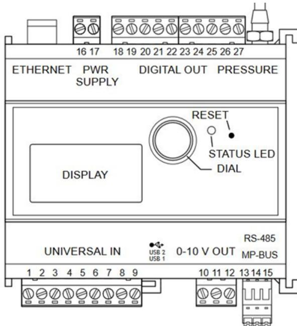
As shown below in the following image the display shows the current status of the controller in this case it can show a serial number of the controller, the current communication configuration, percentage of memory usage, current internal voltage of the controller.
