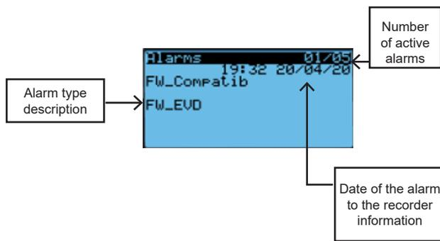
To reset one or all alarms, go to the end of the list on the next screen and press △ for 3 seconds.
