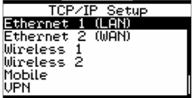
Once the previous menu is selected, the network address of the device can be accessed, as can be seen in the following image, there are different options to which the device has to be adapted depending on the network installation needs or remote monitoring requirements of either the device itself or a third party device such as PC'S, Tablets, or mobile devices.
