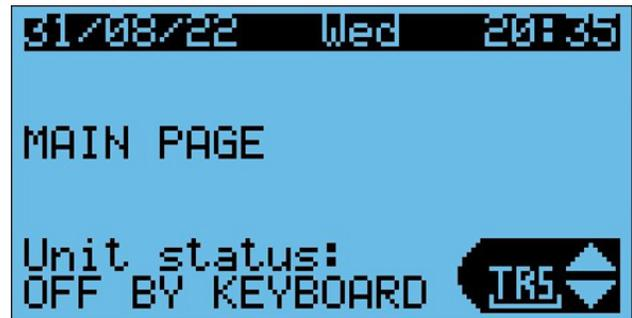
To select the display of the pressure transducers, simply access the menu at the bottom of the screen using the navigation buttons and select the option with the description TRS as shown in the following image.
