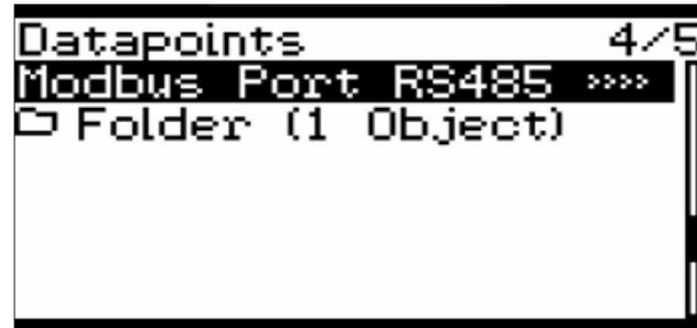
Each menu has a number at the top of the screen, this number indicates the current position of the menu to which you want to access, in this case the parameters to which you want to access is number 4.
