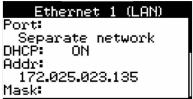
In the following image you can see that selecting the DHCP option in ON mode means that the device can connect to a router that can provide an automatic IP address, depending on whether this router has an Internet connection the device acquires the IP that the router or the Internet connection provides.
