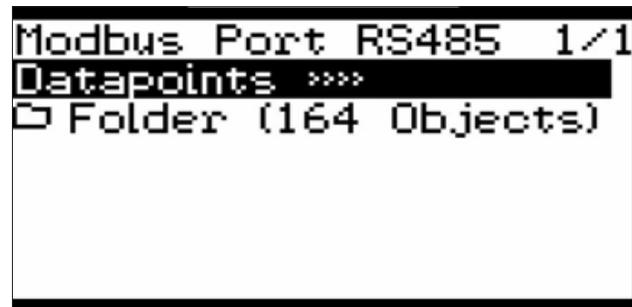
After pressing the dial as shown below and as discussed in the previous step, you will be able to access and observe the values to which the Modbus points are referenced to the communication with the CPCO control.
